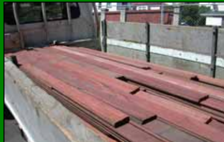
Jarrah flooring recovered for reuse from St Joseph's Church
