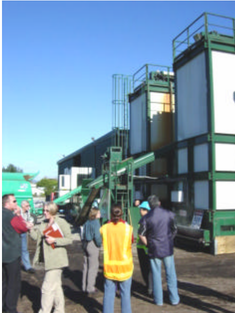
Perrys Environmental 10 Chamber Vertical Compost Uni at Waitakere City Council's resource recovery centre
