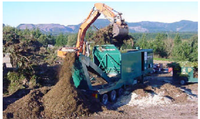
The ripper converts green waste to hog fuel
